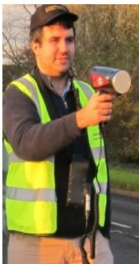
Robert Quarmby uses a radar gun at a spot speed check
